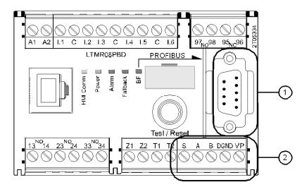
The figure shows the LTMR front face with the PROFIBUS DP connectors:
