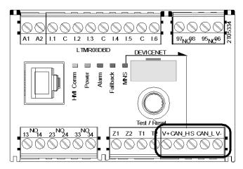
The DeviceNet communication drivers are powered internally.
