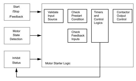
Once the Start or Stop input command is received, the motor starter logic validates the input source. Based on the selected operating mode, the Start or Stop command is performed. The motor starter logic checks the pre-start conditions (inhibit status and motor status). Depending on the selected starter type, the motor starter logic runs the control logics and updates the contactor control output and the inhibit status.
