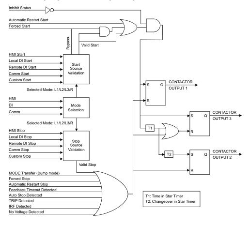
The following diagram shows the logical diagram of the Star Delta starter:
