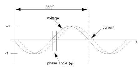
After the phase angle ( $\phi$ ) is measured, the power factor can be calculated as the cosine of the phase angle ( $\phi$ )-the ratio of side a (active power) over the hypotenuse h (apparent power):
