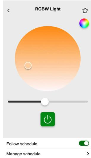
RGBW is controlled by two channels: RGB and W. Tap the circle in the top right corner of the control screen to switch between the RGB and W channels.
