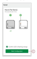
After a few seconds, a solid green LED indicates that the device is successfully paired to the Gateway/Hub.
