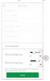
**NOTE:** The Dimming range is limited if the min. and max. levels are too close to each other.
