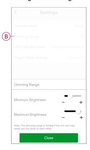
**NOTE:** The Dimming range is limited if the min. and max. levels are too close to each other.
