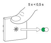
Short press the push-button of the Dimmer 5 times in quick succession.The status LED blinks green.
