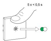
2. Remove the knob and short press the push button 5 times in quick succession.
