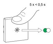
2. Short press the push-button of the Relay Switch 5 times in quick succession. The status LED blinks green.
