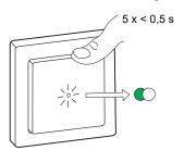
The light connected to the Relay Switch blinks for a few times. The status LED stops blinking green on the Wireless switch and the Relay Switch. The Relay Switch can now be controlled by the Wireless switch.
