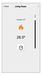
**IMPORTANT:** Once the boost time is set, the set-point temperature automatically increases by 2° C for the set boost time. After the boost time is over, the set-point temperature returns to the current scheduled event or to the previous set-point temperature.
