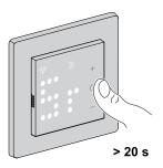
**NOTE:** To cancel the soft reset, press and hold the **O** button for > 30 s. This reverts the thermostat's UI back to its previous state before the touch button is pressed, with no change in a functional state.
