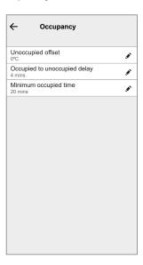
• **Unoccupied Offset**: You set the setpoint when room is unoccupied. This helps to save energy by allowing the temperature to drift from the normal setpoint to a less comfortable but more energy-efficient level when the space is not in use.
