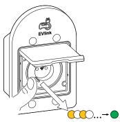
Make sure the LED blinks amber. It takes few seconds for the device to join.
