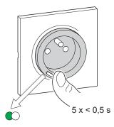
Upon successful pairing, the green LED on the Wireless switch and the Socket Outlet will stop blinking.
