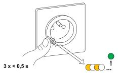
Wait for a few seconds until the LED turns green and the app confirms that the device is joined.
