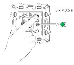
Short press the push-button of the Socket outlet 5 times in quick succession. The status LED blinks green.
