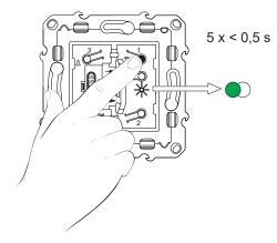
Short press the push-button of the Dimmer 5 times in quick succession. The status LED blinks green.
