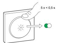
The light connected to the Push-button Dimmer blinks for a few times. The status LED stops blinking green on the Wireless switch and the Push-button Dimmer. The Push-button Dimmer can now be controlled by the Wireless switch.
