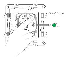
Short press the push-button of the Socket outlet 5 times in quick succession. The status LED blinks green.
