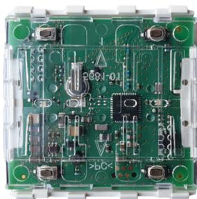
System M: Connected Taster-Modul, 1-fach
