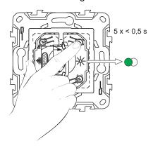
3. Short press the first blind control switch 5 times in quick succession. The status LED blinks green.
