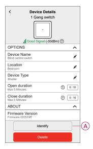
The status LED blinks red and the shutter opens/closes gradually, upon successful identification of the blind control switch or shutter slat.
