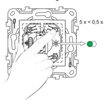
Short press the first blind control switch 5 times in quick succession.The status LED blinks green.
