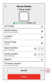
The status LED blinks red and the shutter opens/closes gradually, upon successful identification of the blind control switch or shutter slat.
