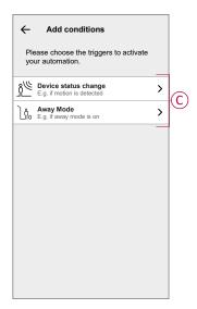
a. In this example, we will select **Device status change** and choose a device to set the condition. Then, we will select the state of the device that will trigger the automation, such as the closed state of a blind control switch.
