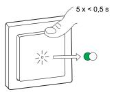
The light connected to the Push-button Dimmer blinks for a few times. The status LED stops blinking green on the Wireless switch and the Push-button Dimmer. The Push-button Dimmer can now be controlled by the Wireless switch.
