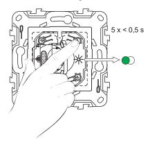
3. Short press the push-button of the Dimmer 5 times in quick succession. The status LED blinks green.
