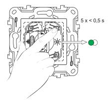
3. Remove the knob and short press the push button 5 times in quick succession.
