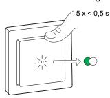
The light connected to the Push-button Dimmer blinks for a few times. The status LED stops blinking green on the Wireless switch and the Push-button Dimmer. The Push-button Dimmer can now be controlled by the Wireless switch.
