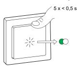
The light connected to the Relay Switch blinks for a few times. The status LED stops blinking green on the Wireless switch and the Relay Switch. The Relay Switch can now be controlled by the Wireless switch.
