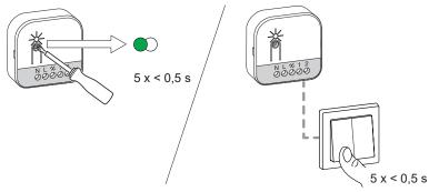
The light connected to the Dimmer blinks for a few times. The status LED stops blinking green on the Wireless switch and the Dimmer. The Dimmer can now be controlled by the Wireless switch.
