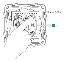
Short press the push-button of the Relay Switch 5 times in quick succession. The status LED blinks green.
