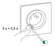
Upon successful pairing, the green LED on the Wireless switch and the Socket Outlet will stop blinking.
