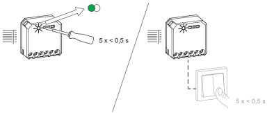
The shutter moves up and down for a few times. The status LED stops blinking green on the Wireless switch and the Puck. The Puck can now be controlled by the Wireless switch.
