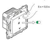
The shutter will move up and down a few times. When successfully paired, the status LED on the Wireless switch and the blind control switch turns Off.
