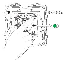
Short press the push-button of the Dimmer 5 times in quick succession. The status LED blinks green.
