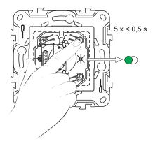
3. Short press the push-button of the Socket outlet 5 times in quick succession. The status LED blinks green.
