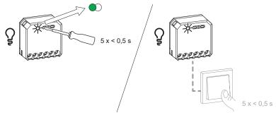
The light connected to the Puck blinks for a few times. The status LED stops blinking green on the Wireless switch and the Puck. The Puck can now be controlled by the Wireless switch.
