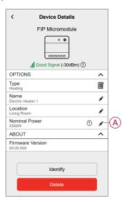
Tap **OK** and enter a value between 1 to 4600 W based on the load connected. The settings will be saved automatically.
