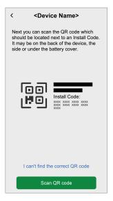
NOTE: If the dimmer doesn't have the QR code or MAC Address and Install Code, you can manually pair it by tapping I can't find the correct QR code
