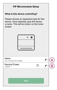
11. Tap **OK** and enter a value between 1 to 4600 W based on the load connected.
