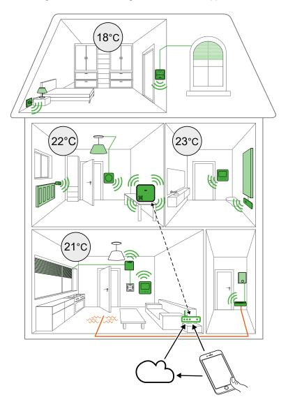
The Hub is the center of the system, processing control requests and status reports for connected Wiser devices, page 13.
