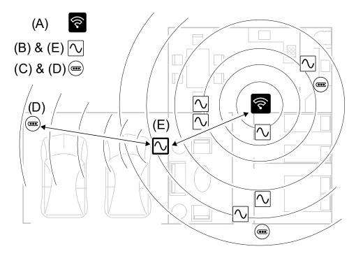
**TIP:** The **battery-powered motion sensor** in the **garage** (D) is a long way from the Hub. However, the sensor can connect to the hub via the **main-powered device** being used as the **garage light switch** (E). This is because mains-powered devices also act as system network extenders. Consider this when deciding where to locate the Hub.
