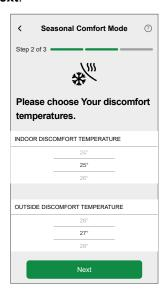
**NOTE:** Discomfort temperature refers to a temperatures above which an individual feels uncomfortable. When the ambient temperature raises above the set inside and outside discomfort temperatures, the seasonal comfort mode closes the shutters to maintain the indoor temperature. Maintaining a comfortable indoor temperature helps improve well-being and productivity.
