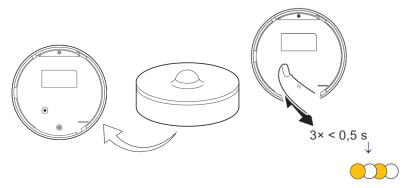
Wait for a few seconds until the LED turns green and the app confirms that the device is joined.
