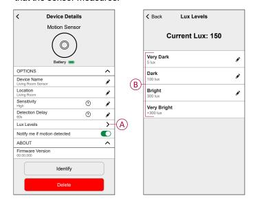
**NOTE:** In the sensor, the lux value is predefined by default. However, you can change the lux value using the sliding bar; for example, see **Very Dark**.
