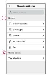
Devices (J): Select a device from the list and set the device status (e.g., ON/OFF, delay). Then, tap Done.
