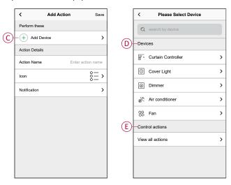
Devices (D): Select a device from the list and set the device status (e.g., ON/OFF, delay). Then, tap Done.
